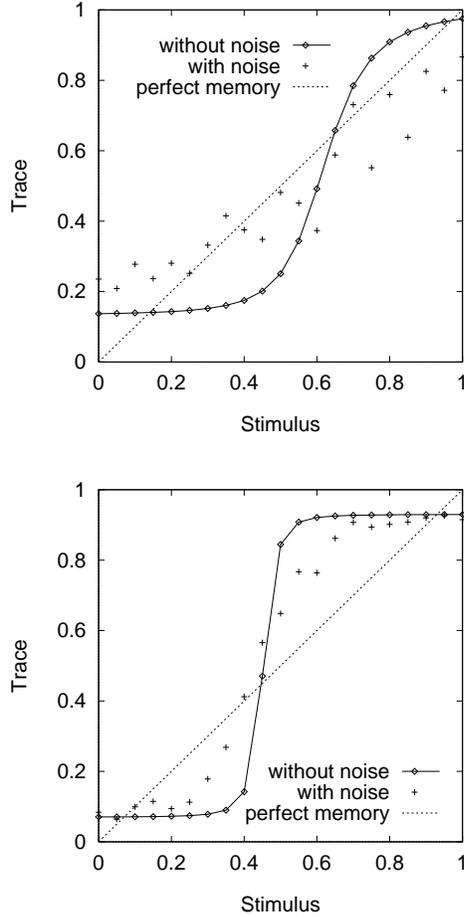
Figure 3: Memory response of the Zipser model at time step 10 (top) compared with the memory response of the single unit sigmoid model at time step 7 (bottom). Each hatch mark shows the noisy response to a fixed stimulus. For comparison, the diagonal line (stimulus = trace) shows perfect memory.
