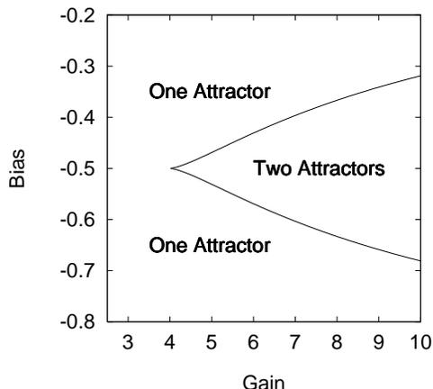
Figure 2: Bifurcations in the dynamics of the single unit sigmoid model as a function of the gain and bias parameters.
